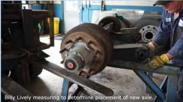
Billy Lively measuring to determine placement of new axle.
