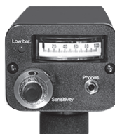
For air leak detection, ESCO uses this handheld ultrasonic device, which is mfg. by UE Systems, Inc.
